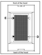
Install charcoal filter (plastic side exposed) into charcoal filter bracket. Insert tab cut-out side D of charcoal filter into bracket first. Lock charcoal filter into place by pushing down on side E with locking tabs.
